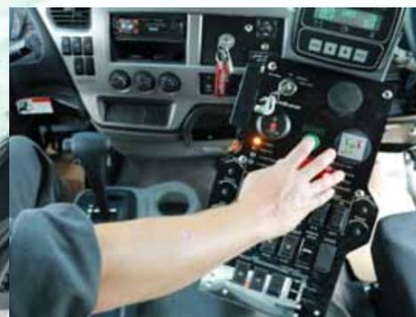
*The console is conveniently located between the operator stations. A single-button Start/Stop System allows the driver to operate sweeper functions without looking at the control panel.*
